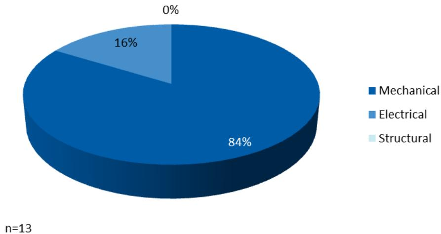
Electrical failures were the second-most common cause of system downtime. Five projects (28%) reported electrical failures resulting in an average downtime of three months—three WTIC, one Seaforth, and one Southwest wind turbine. We estimate that electrical failures accounted for 16% of total downtime reported.
