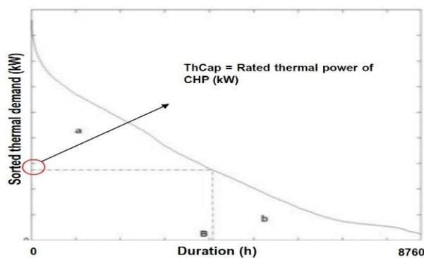
Figure 8-load-duration diagram - Biggest rectangle method for CHP sizing
